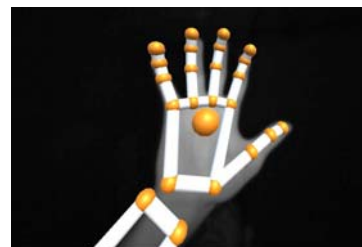
Fig. 2. Recognized points of the hand in Leap Motion
